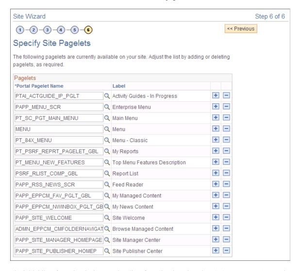
The initial list of pagelets is the complete list of pagelets based on the PS\_SITETEMPLATE registry. All pagelets are initially assigned to new sites. You can add or delete pagelets as required.
