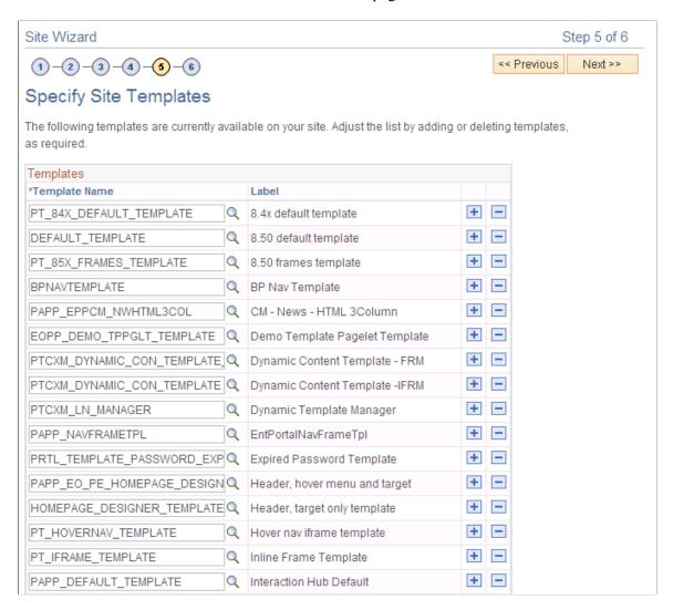
This initial set of templates is the complete list of available templates based on the PS\_SITETEMPLATE registry. All templates are initially assigned to new sites. You can add or delete templates as required.
