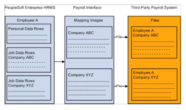
This diagram shows how company filtering maps an employee's company data into separate files.
