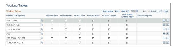
The tables listed in the **Record (Table) Name** column are the records and tables to which you can grant (or deny) SQL access. Although we have predefined access to many tables in the Time and Labor system, you can change the delivered settings and can insert new rows for additional tables that you must access within your rules. All tables in the HCM system are available for rules development. The only tables you do not have access to are PeopleTools tables.
