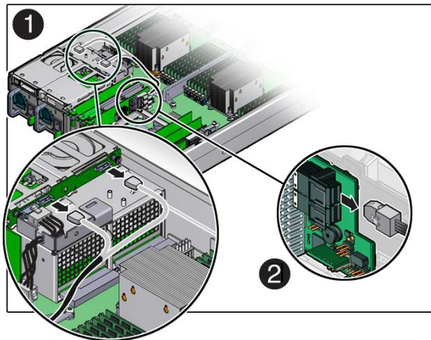
4. Install the replacement SAS cable to the rear disk drive backplane [1] and the SAS card [2] as shown in the following figure.
