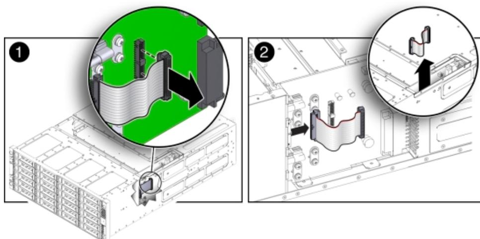
4. Disconnect the HDD ribbon cable connector located on the disk midplane module [2] as shown in the previous figure.
