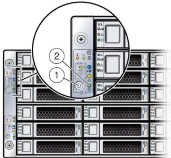
On the server node, the green Power/OK LED (see [2] in the previous figure) blinks while the server node is booting, and remains steady on when the server node is operational.
