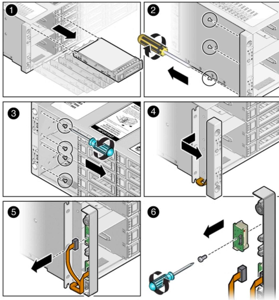
3. Unscrew the three Phillips screws from the back of the ear bezel [2] as shown in the previous figure.
