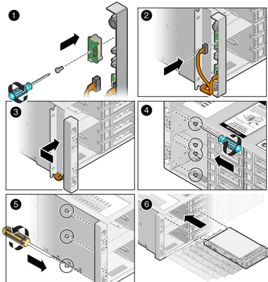
2. Connect the ribbon cable to the indicator panel [2] as shown in the previous figure.
