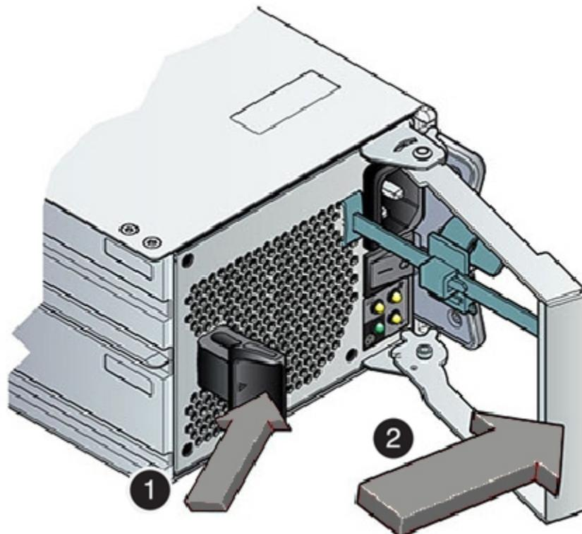
4. Install the replacement power supply unit using the procedure for your storage shelf model:
