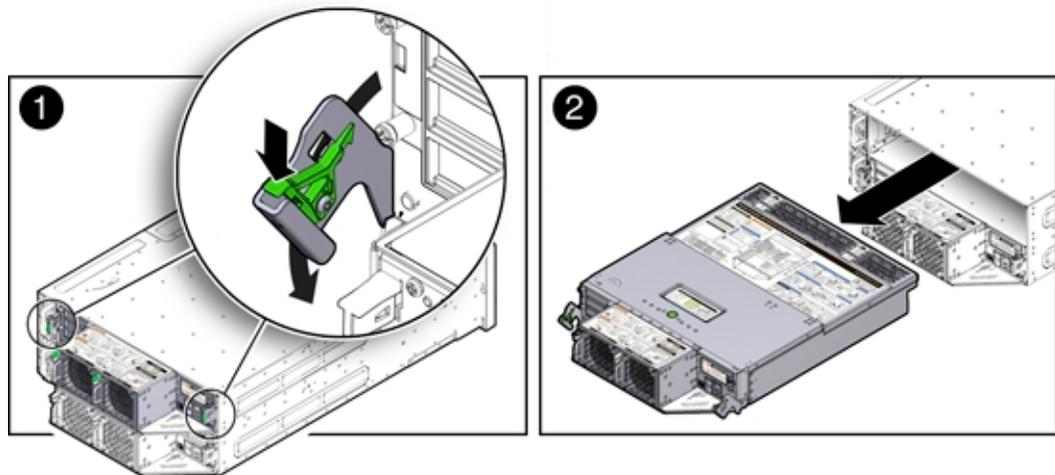
3. Slide the server node to the rear and lift it out of the system [2] as shown in the previous figure.
