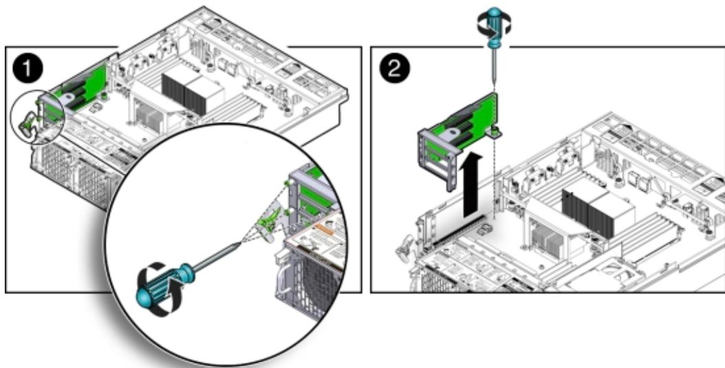
6. Loosen the green captive Phillips screw that secures the PCIe riser to the motherboard [2].
