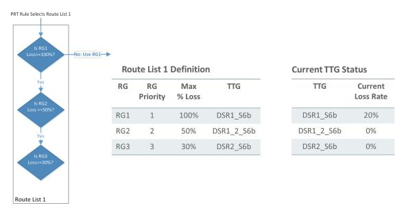
The next figure shows what happens when none of the Route Groups meets their minimum threshold. In this case all three Route Groups are skipped, and the action defined in the new "Routing Congestion Action" in the Routing Option Set is executed. Like the other actions defined in the ROS, this new action can either abandon the answer, or return a user-configured
