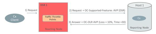
When the Host decides that it needs to reduce the traffic being sent to it, it includes (piggybacks) an OC-OLR AVP in an answer to a request message that included the OC-Supported-Features AVP. The OC-OLR AVP includes:
