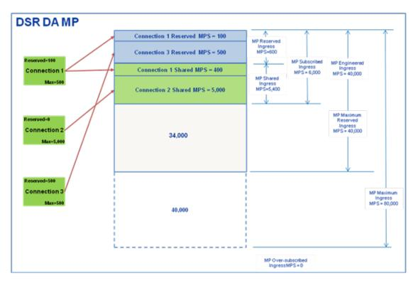
The DSR prevents the total Reserved Ingress MPS of all connections hosted by a DA MP from exceeding the DA MP's maximum ingress MPS. The enforced limit for this is the DA MP's licensed MPS capacity, which defaults to the DA MP's maximum engineered capacity. The enforcement of this requirement on 'configured' connections versus 'Enabled' or 'Active' connections is a design decision.
