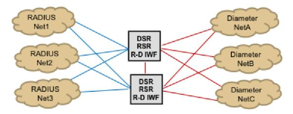
As shown in the above figure, Diameter transport is planned for the 'c-links' between DSR mates, even forRADIUS messages. This is possible because RADIUS messages are encapsulated within a Diameter shell forinternal routing within a DSR.
