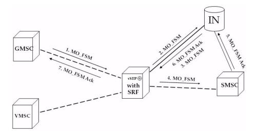
The Gateway Mobile Switching Center (GMSC) sends the Mobile Originated Forward Short Message (MO\_FSM) to the vSTP with PPSMS (TCBEGIN). Based on MTPDPC = vSTP point code and SCCP CdPA TT, NP, NAI, SSN, and GTI, the message is pre-selected for PPSMS service. If service is not PPSMS, the message falls through to GTT.
