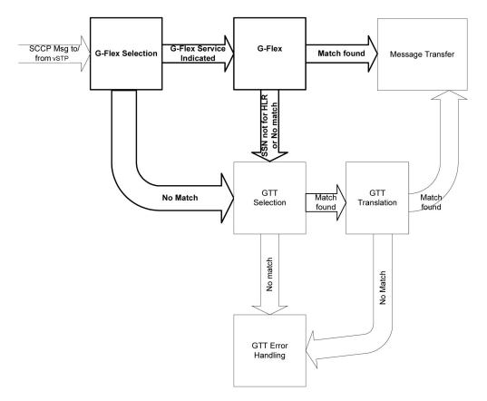
In order to keep the diagram simple, the only error conditions shown are the no-match cases for G-Flex and GTT selectors and translations. G-Flex has its own error handling for some cases that issues measurements and peg measurements appropriately before letting the MSU fall through to GTT translation. Also, there are error conditions in GTT selection, GTT translation, and message transfer that are handled by GTT error handling.
