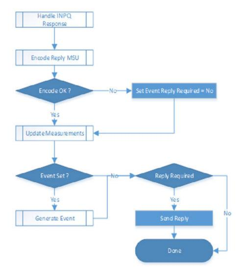
Figure 2-18 INPQ Function Flow Chart - Sheet 3 of 3
