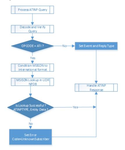
Figure 2-13 ATI NP Function Flow Chart - Sheet 2 of 3
