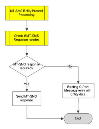
Figure 2-2 G-Port SMS-MT Processing for Entity Found Case
