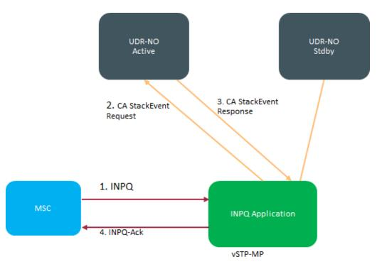
Figure 2-15 Message Flow for INPQ Solution on vSTP
