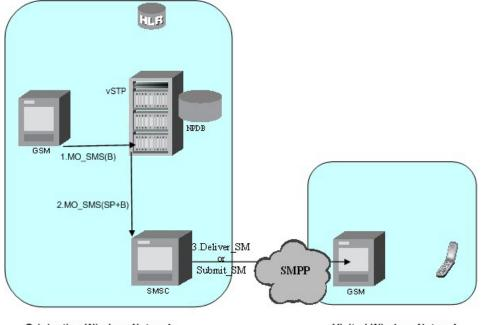
Figure 5-10 MO-Based GSM SMS NP Call Flow for Other-Network Subscriber
