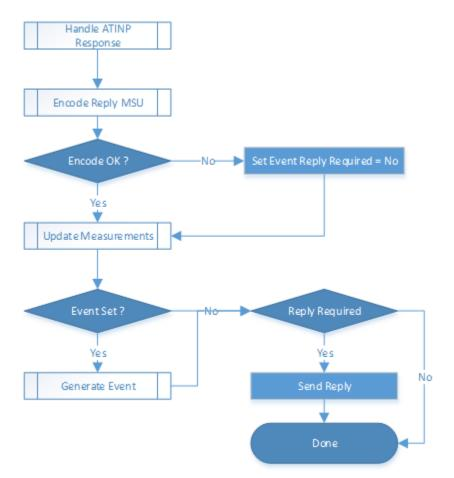
Figure 2-14 ATI NP Function Flow Chart - Sheet 2 of 3
