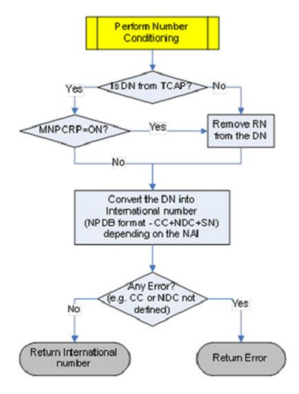
Figure 2-5 G-Port Number Conditioning Flowchart
