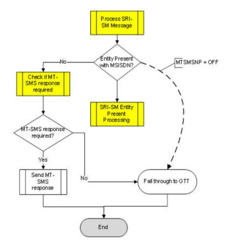
Figure 2-1 G-Port SMS-MT Processing for No Entity Case
