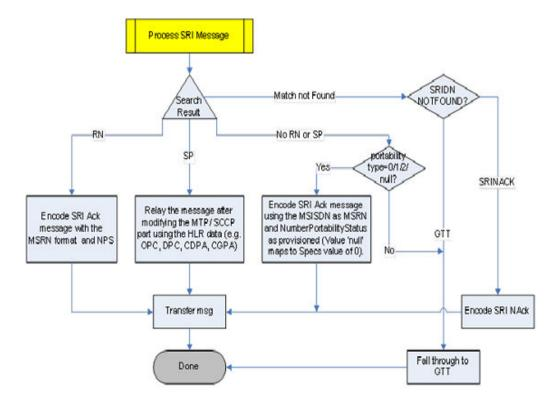
Figure 2-9 G-Port SRI Processing Flowchart
