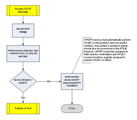
Figure 2-3 vSTP MNP G-Port Function Flowchart - Sheet 1 of 2
