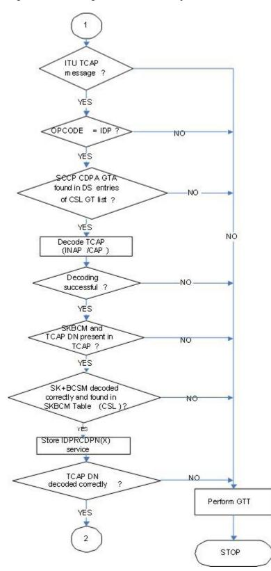
Figure 5-2 Message Flow for IDP Relay - Sheet 2 of 3
