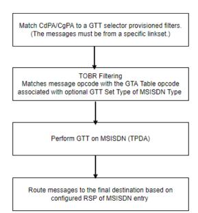
Figure 2-17 Call Flow of TPDA Based Filtering
