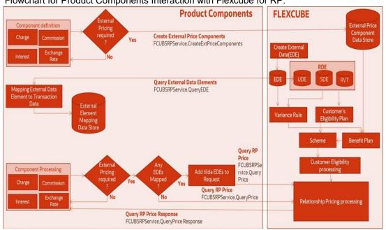
Flowchart for Product Components Interaction with Flexcube for RP.
