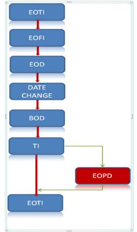
The below flowchart indicates the EOD process in the system.
