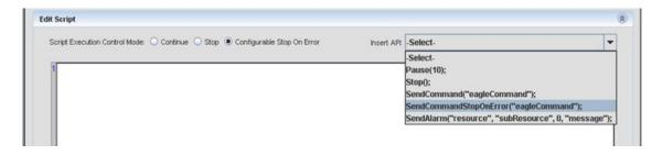
The **Script Execution Control Mode** radio buttons are available on the Create Script and Modify Script screens to control script behavior when a command fails on the EAGLE. The three possible behaviors are:
