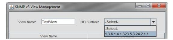
After adding the **View Name** and selecting the **OID Subtree**, click **Add** to create the new SNMP v3 view. A notification is provided in the system tray and the new view is added to the view list on the SNMP v3 View Management screen.
