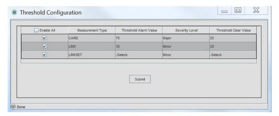
2. Enable each Measurement Type within the check box or Enable All check box on the column header. By default, the check box on the column header and for all the three rows are unchecked i.e., the thresholding functionality is disabled for all the measurement types.
