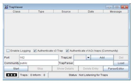
9. Change the **Port** field to the port where SNMP v3 traps are expected from OCEEMS and then click **Start**.
