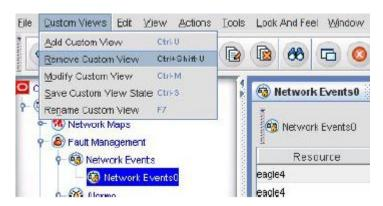
Right-click on the custom view node under the Network Events/Alarms node in the left navigation pane, and choose Custom Views, and then Remove Custom View as shown in Figure F-13.
