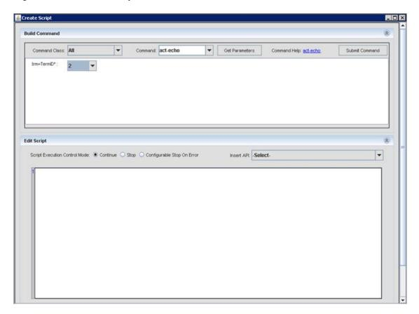
While creating command scripts, for command parameters with values that need to be specified in double quotes, you must use the backslash (\) character before each double quote to be able to save the script successfully. For example, to include the following command in a script:
