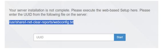
12. Log in with the non-root user and go to **i-net installation directory**. Run the following commands to view the contents of webconfig.txt file. Get UUID from webconfig.txt.
