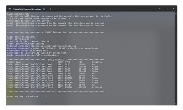
Upon clicking the Shelf View, no further action is required. On clicking it, a terminal window will open and it will display the ALARM severity status of each card on the shelf. When you click it for the first time, it will pop up automatically. Upon clicking the Shelf View subsequently, you must manually refresh the view to display the pop up with the most up-to-date information. To refresh the view, click the refresh button.
