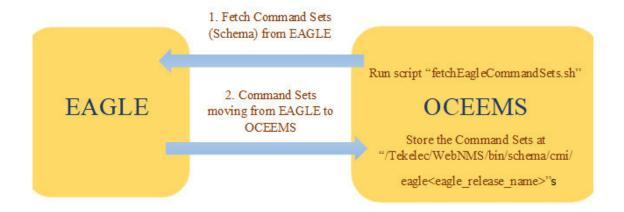
Before installing the CMI schema (command set) of a specific EAGLE release, the CMI schema of that specific EAGLE release must be present in OCEEMS at /Tekelec/ WebNMS/bin/schema/cmi/eagle<eagle\_release\_name>. If the respective CMI schema is not present in OCEEMS at the previously mentioned filepath, then installE5MSSchema.sh will not be able to install the CMI schema (command set) of that specific EAGLE release.
