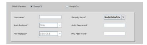
The following fields are required when the SNMPv3 radio button is selected:
