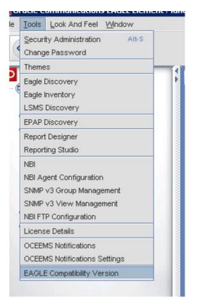
The current compatible EAGLE release or version with the OCEEMS means that the OCEEMS is supporting the schema or command set of the displayed EAGLE release, with which it is currently compatible:
