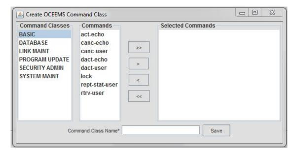
Locate commands to be added to the custom command class by selecting a command class in the Command Classes pane on the left, selecting one or more commands from that command class from the Commands pane in the middle, and then using the arrow keys to move commands to the Selected Commands pane, as shown in Figure 11-28.
