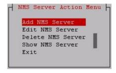
On the Add an NMS Server screen, enter/select values for the OCEEMS Name, IP address, Port, and SNMP Version fields. For v3 specify the HeartBeat and User fields, and for v1 specify the SNMP Community String field.
