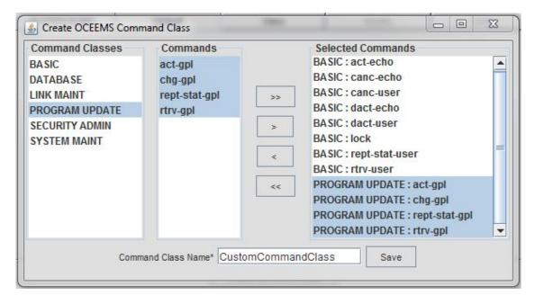
You can locate and select commands from multiple command classes to be included in the custom command class. In Figure 11-28, all commands from the BASIC and PROGRAM UPDATE command classes were selected.
