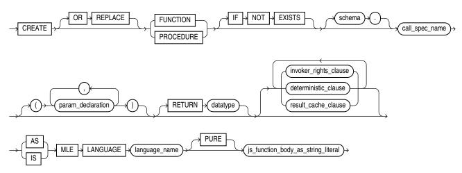
Figure 6-5 MLE Inline Call Specification Syntax
