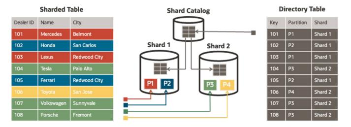
Key insert and update operations are performed on the shard catalog, and synchronously duplicated to the shards at commit time.
