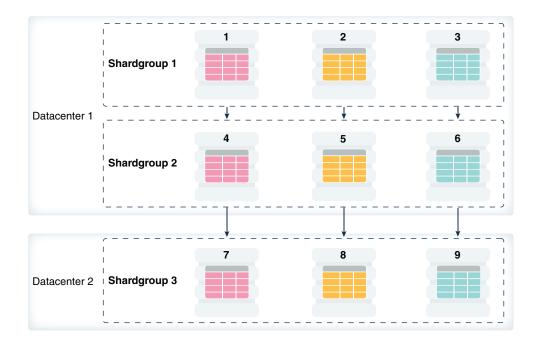
Figure 5-1 System-Managed Sharding with Data Guard Replication
