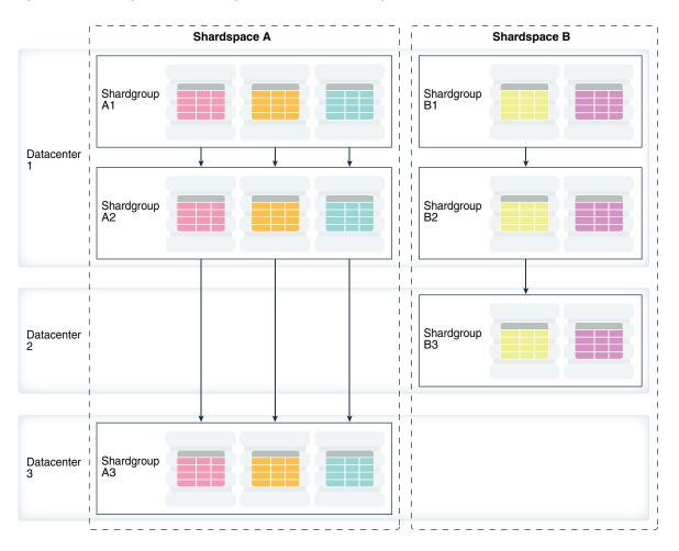
Figure 5-3 Composite Sharding with Data Guard Replication
