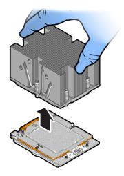
5. Place the heatsink, facing up, on a work surface.
