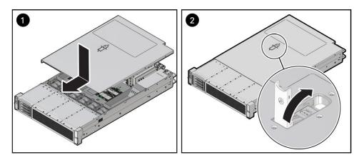
Latch the top cover closed by pushing down on the button until it is flush with the cover and you hear an audible click [2].
