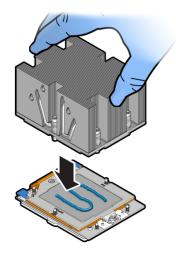
Using torque driver set to 12 in-lb (13.5 kg-cm) to 13.02 in-lb (15.0 kg-cm) force with a Torx T20 bit, tighten the heatsink module to the socket as shown in the following illustration. Note that screws 1 and 2 are slightly longer than screws 3, 4, 5, and 6.
