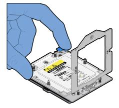
Lift the processor rail frame by holding its lift tabs and rotating the rail frame to its near vertical position.
