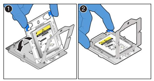
c. Rotate the force frame to its closed position on the socket stiffener frame.
