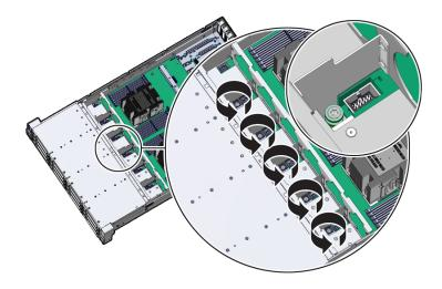
4. When removing the fan tray, slightly tilt the fan tray to the left to decompress the cables, before removal.
