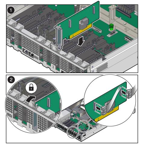
If it is difficult to reconnect the cables to the PCIe card when the card is inserted into the PCIe slot, consider performing the procedure in Step 5 before completing this step.
