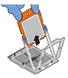
**12.** Place the carrier frame package in an appropriate tray.
