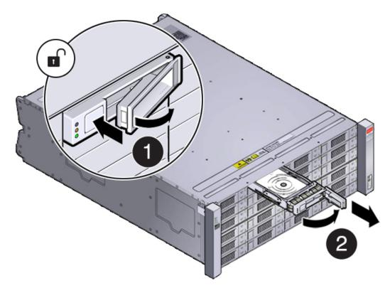
3. Install the replacement drive by opening the drive lever on the replacement drive. Slide the new drive into the drive slot [1] until it engages with the backplane connector and then
