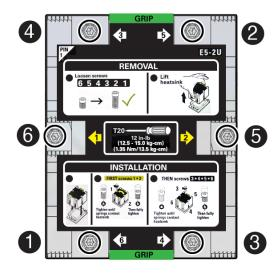
4. Lift the heatsink from the socket.
