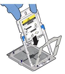
Ensure that the two insertion tabs at the bottom of the External Cap are inserted into the slots in the rail frame.
