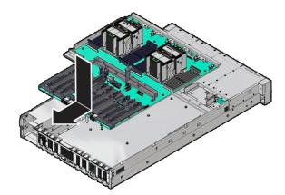
**3.** Using a Torx T25 screwdriver, tighten the two captive screws to secure the motherboard mid-wall to the chassis.
