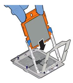
Ensure that the two insertion tabs at the bottom of the processor carrier are inserted into the tab slots in the Rail Frame.
