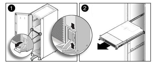
4. While the release latch covers are in the open position, slowly pull the server forward until the slide-rails latch into a locked position [2].
