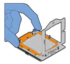
**11.** Lift the Rail Frame and slide out the carrier frame package.
