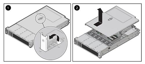
4. Lift up and remove the top cover [2].
