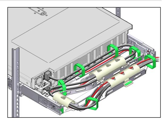
**13.** Ensure that the secured cables do not extend above the top or below the bottom of the server to which they are attached.
