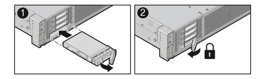
6. Power on and remount the replacement drive. Type the following command from the host:
