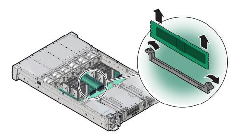
4. Replace each failed DIMM with either another DIMM of the same rank size (quad-rank or dual-rank) or leave the slot empty.
