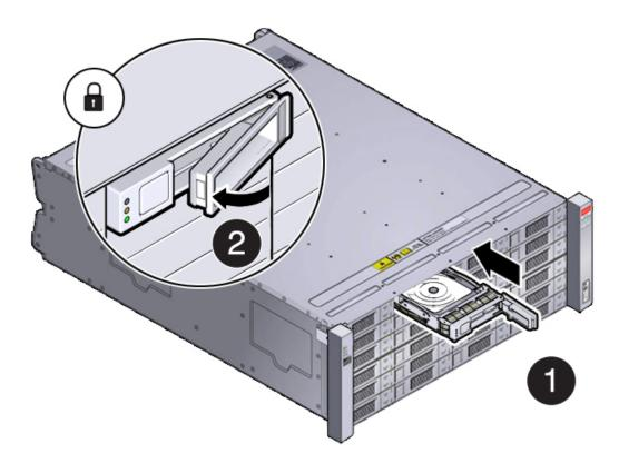
4. Once installed, the system should automatically detect and use the replacement drive. Ensure that the green OK indicator for the replacement drive lights to show that the drive is ready.
