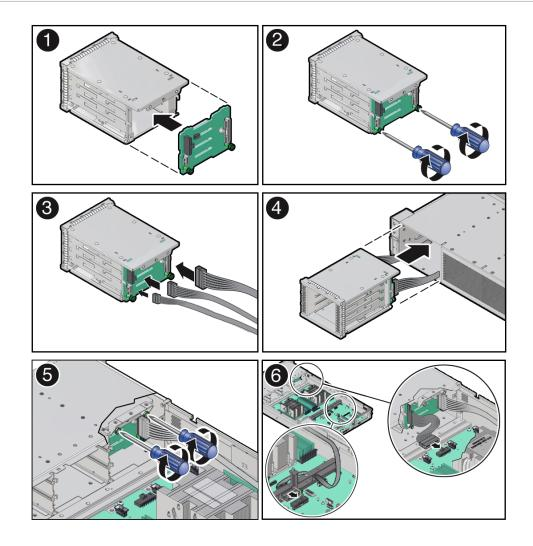
b. Reconnect the disk backplane cables to the disk backplane [3].
