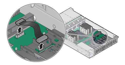
At each end of the cable, press and hold the metal clip to disengage the locking mechanism, then gently lift the PCIe Flyover cable from the connector.
