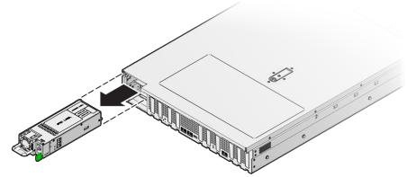
7. Pull the power supply out of the chassis.
