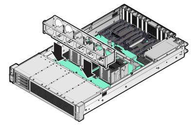
Ensure all motherboard cables are clear of the fan tray and fan tray gasket.
