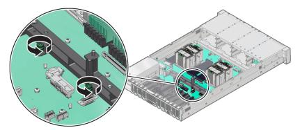
**10.** Remove the motherboard from the server with reusable components that populate the motherboard in place.
