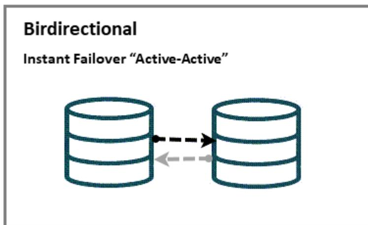
The active-active solution allows data updates and changes ("write" activity) to occur on two or more active databases supporting live applications. Oracle GoldenGate synchronizes the two active databases by replicating the data between each at a logical level and allows load distribution to improve system performance. In the case of an outage of one system, there is no downtime for the end user because the other active system continues with operations.
