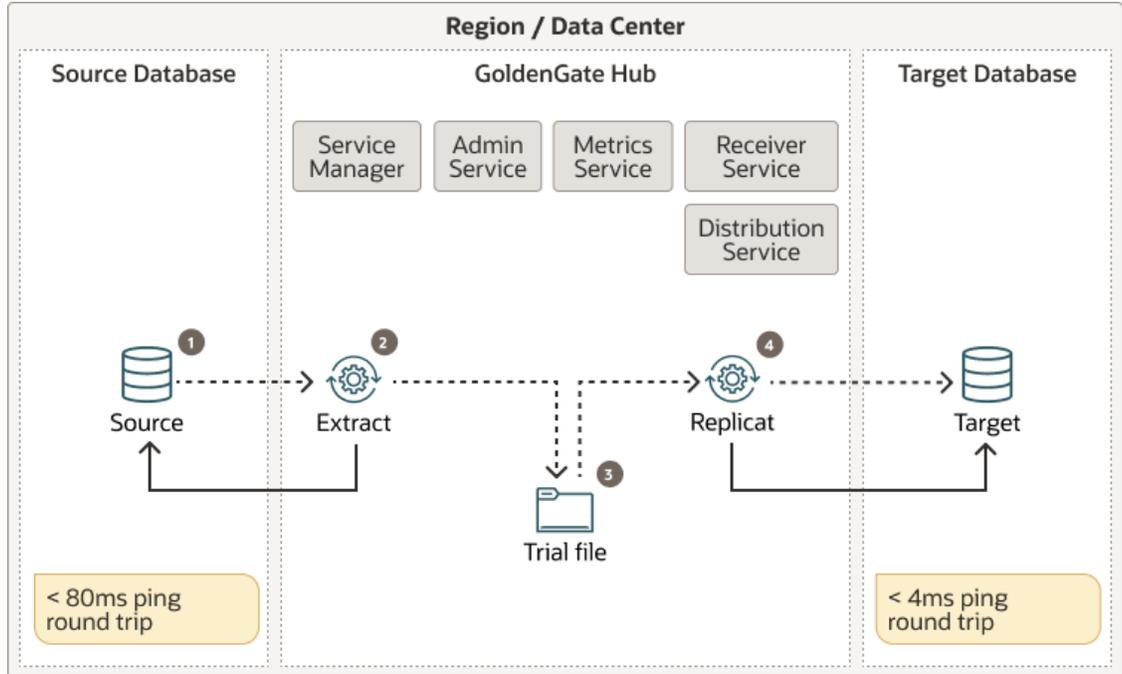
This configuration can have multiple Oracle GoldenGate installations with multiple deployments managing a fleet of replication streams with similar or different topologies and use cases.
