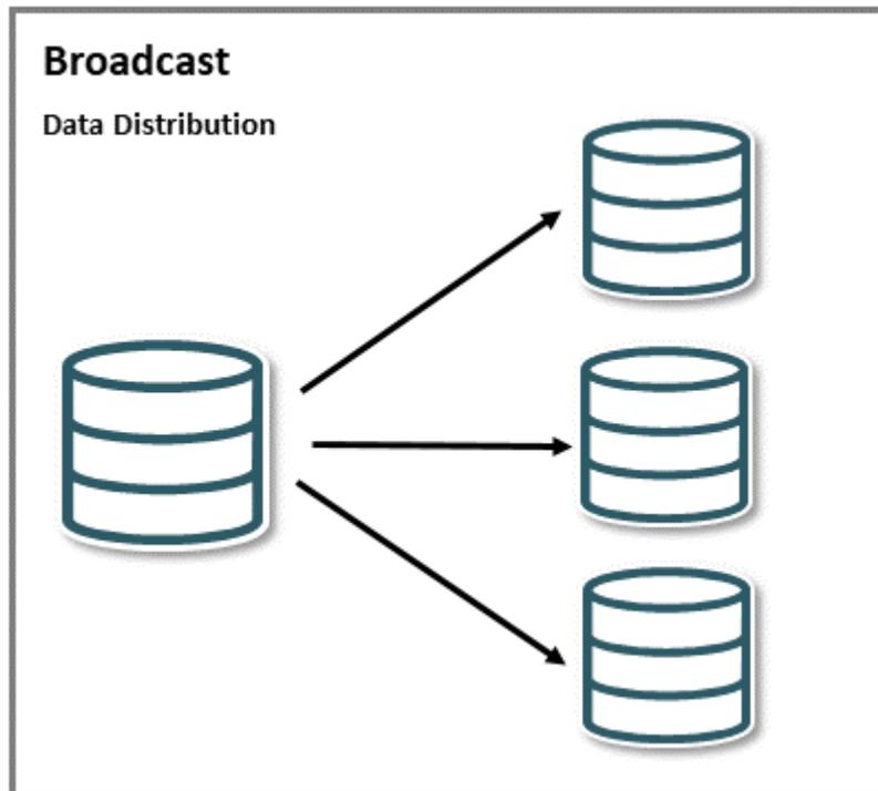
Broadcast topologies can include a mix of unidirectional use cases, including offloading of reporting, replication to a data warehouse, or sending data to a lower level environment. In most cases, administrators configure a single Extract process that writes to multiple trail files. Each trail file is used for a different target database. This reduces the overhead on the source database, and allows each target platform to receive just the data that it requires.
