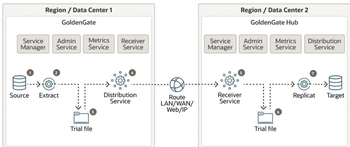
In this diagram, two Oracle GoldenGate deployments are set up on two different database servers, which are connected over the network. Consider, Data Center 1 as the source and Data Center 2 as the target. Both the deployment are local to their respective database server.
