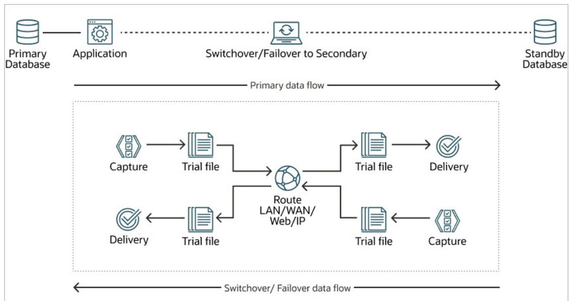
In this configuration, there is an inactive Oracle GoldenGate Extract group and an inactive Distribution Path on the live standby system. Both these groups remain stopped until just before user applications are switched to the live standby system in a switchover or failover. When user activity moves to the standby, those groups begin capturing transactions to a local trail, where the data is stored on disk until the primary database can be used again.
