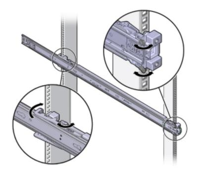
Figure 2-1 Locking the Slide-Rail Assembly Against the Inside of the Rear Rack Rail
