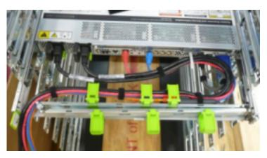
Figure 2-6 Cables Secured under the Cable Clasps
