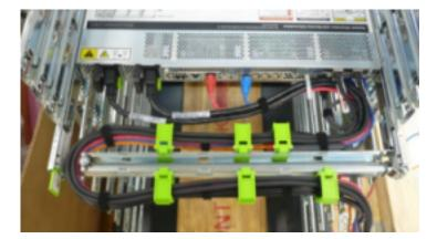
Figure 2-8 RDMA Network Fabric or TwinAx Cables Positioned on the CMA
