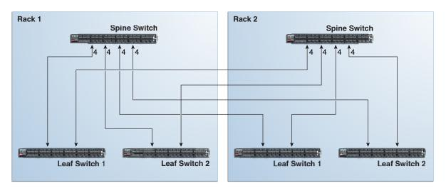
As shown in the preceding graphic, each leaf switch in rack 1 connects to the following switches:
