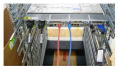
Figure 2-3 Cables at the Rear of the Server
