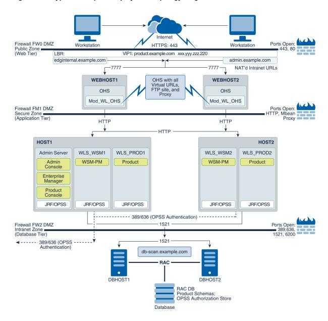
Figure 2-1 Typical Enterprise Deployment Topology Diagram
