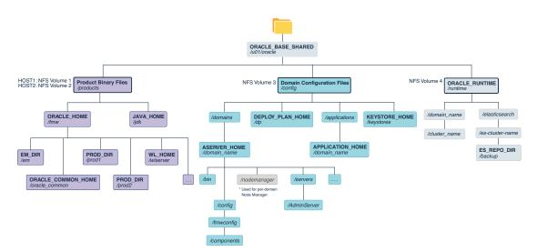
Figure 7-1 Recommended Shared Storage Directory Structure for an Enterprise Deployment
