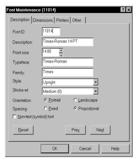
On the Description tab, make sure the settings for the Stroke wt., Style, and Spacing fields are correct. Italic fonts should have a style of *Italic*. Bold fonts should have a stroke weight that's greater than zero. Fixed pitch fonts should have a spacing of *fixed*. And, proportional fonts should have a spacing of *proportional*.
