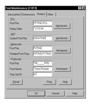
The Printers tab lets you enter printer-specific information for PCL, AFP, Metacode, and PostScript printers. In the AFP (or Metacode) section of the Printers page, the Font File field should contain the name of the font file.
