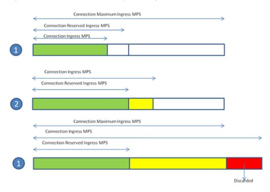
Figure 12-1 Per-Connection Message Coloring
