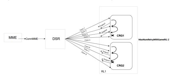
Figure 2-2 Timeout Based Redirection Connection Group
