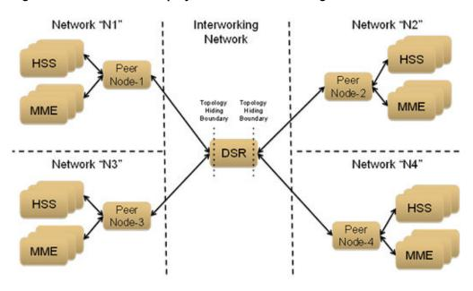
Figure 9-5 TH Network Deployment in an Interworking Network
