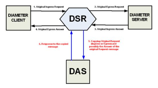
Figure 11-1 Diameter Message Copy Message Flow
