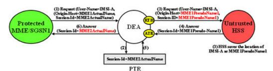
Figure 9-15 MME/SGSN TH Protected-MME/SGSN to Untrusted HSS Transaction
