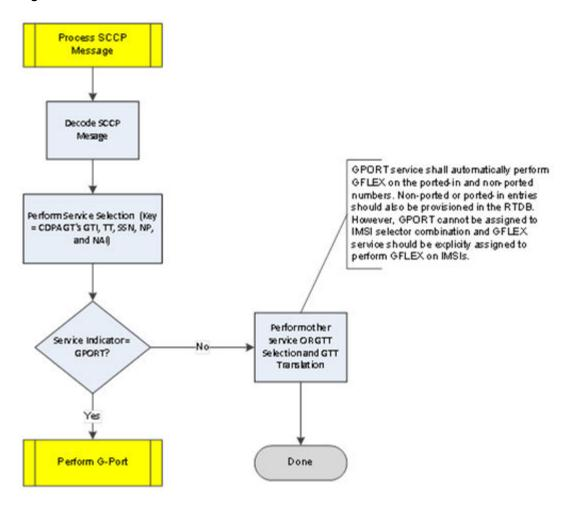
Figure 2-3 vSTP MNP G-Port Function Flowchart - Sheet 1 of 2
