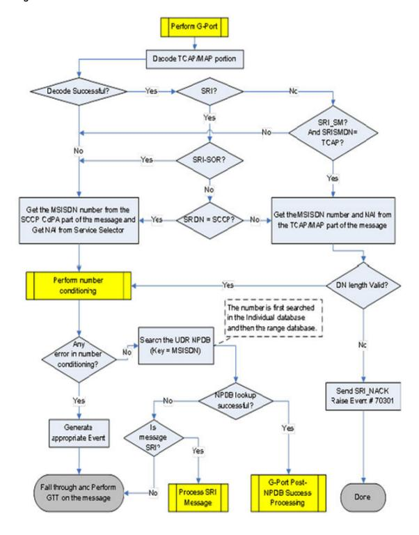
Figure 2-4 vSTP MNP G-Port Function Flowchart - Sheet 2 of 2
