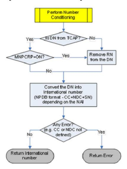
Figure 2-5 G-Port Number Conditioning Flowchart
