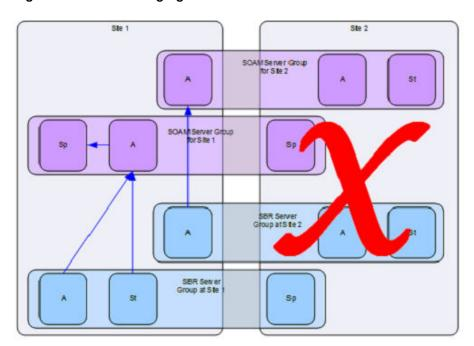
Figure 2-15 Data Merging – Redundant Site Failure
