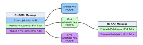
Alternate Keys can be configured with a priority (values 1 through 5, where 1 is the highest Priority (IMSI, IPv4, IPv6, or MSISDN). This improves the chances of finding the data in the Diameter message and the chances of finding the Alternate Key in the Binding database.
