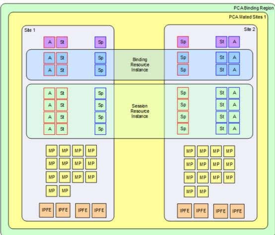
Figure 2-6 illustrates a possible configuration for additional mated pairs that do not host the Binding database:
