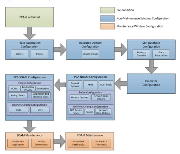
Figure 5-1 PCA Configuration Flow
