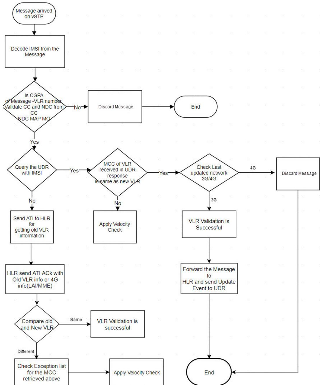
Figure 2-13 Perform Velocity Check
