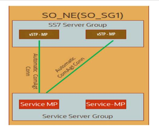
By default, the **vSTPService** process remains OFF. Turn On the **vstpService** process on the service MP to enable the Home SMS Router functionality. To enable the feature, run the following commands:
