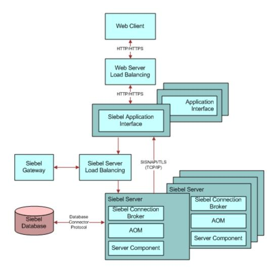
As shown in this diagram, a typical Siebel CRM client request flows from the user's Siebel Web Client through the system, and back again. The general flow is as follows:
