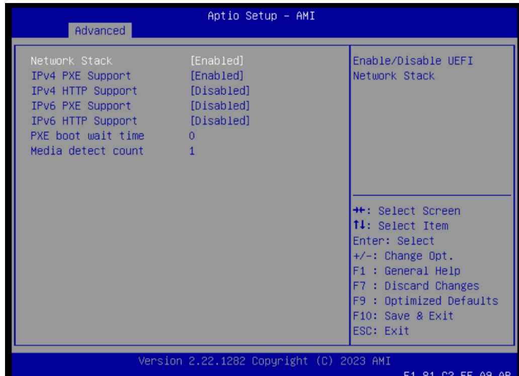
Figure 2-10 Network stack configuration
