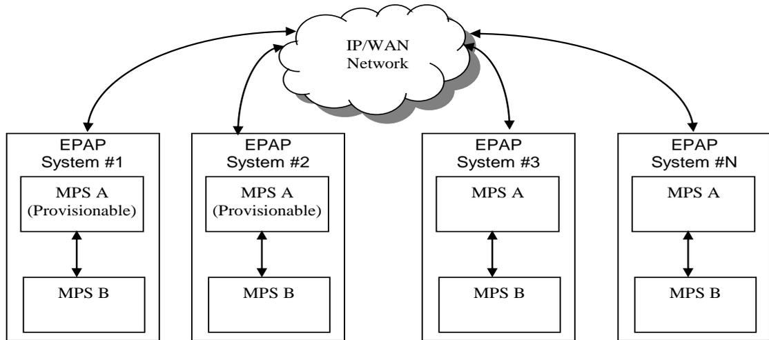
**Figure 5: EPAP Mated Pairs with Non-Provisioning MPS Servers**
