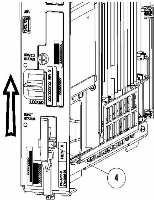
**Figure 6: Slide the Ejector Switch**
