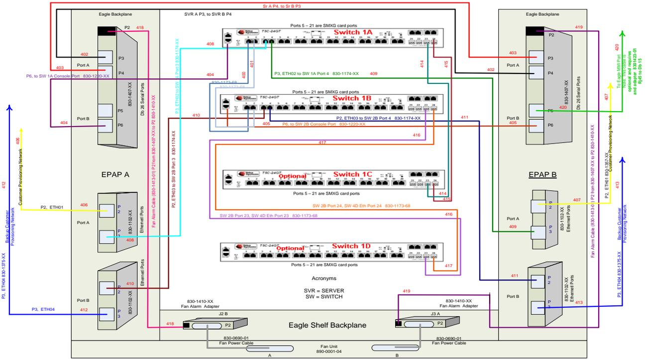
Figure 9: Default Interconnectivity Diagram (Eth04 used for Backup Provisioning Network)
