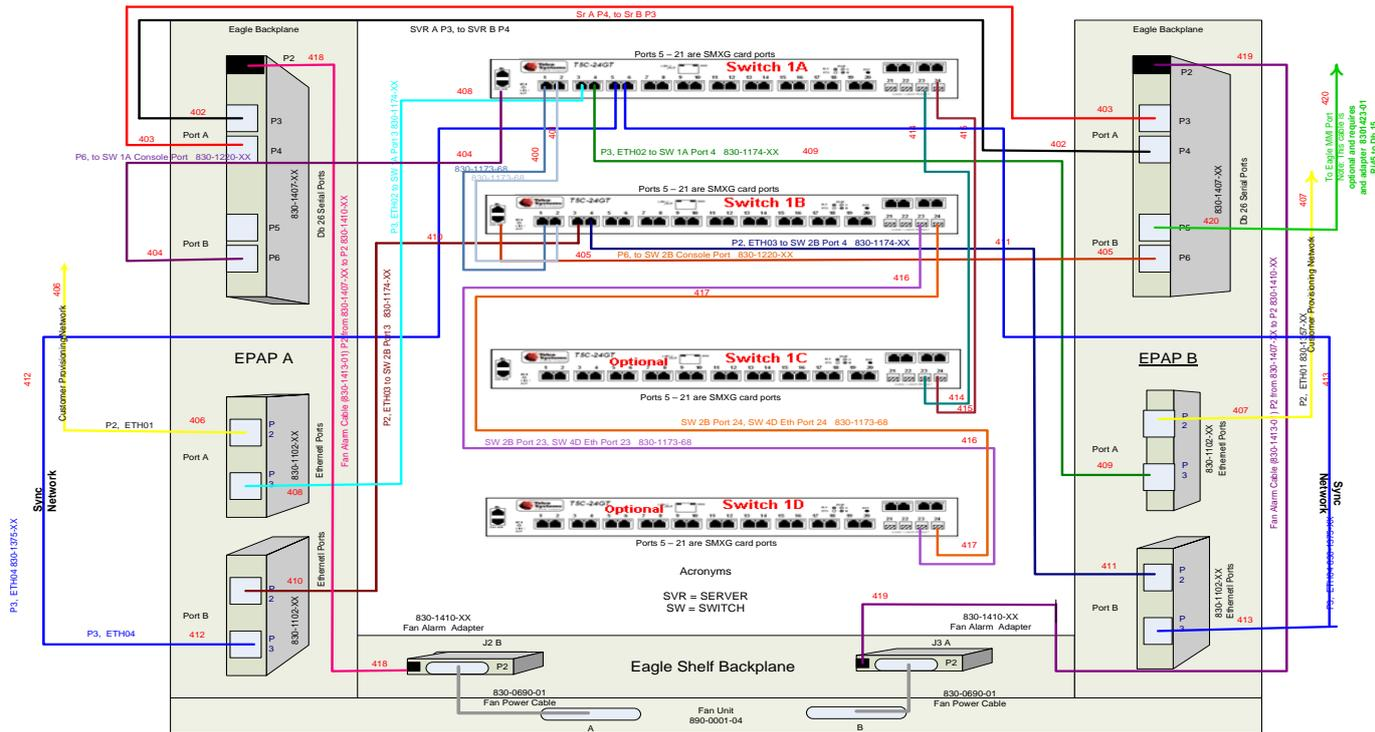
Figure 8: Interconnectivity Diagram for Sync Network Redundancy (Eth04 used for Sync Network)
