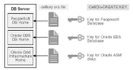
Figure 4-2 Security Keys and cellkey.ora Files
