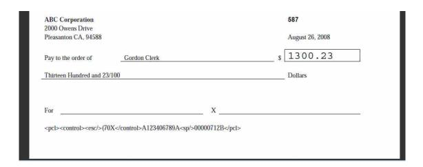
When this PDF is converted to PCL,  $\langle esc \rangle$  is converted to the escape character 0x1b; the PCL command is included from the PDF ((70X);  $\langle sp \rangle$  is converted to a space character and the text is generated with the PCL absolute cursor positioning command (&a#v#h#P). The following figure shows the PCL output displayed using a text editor.
