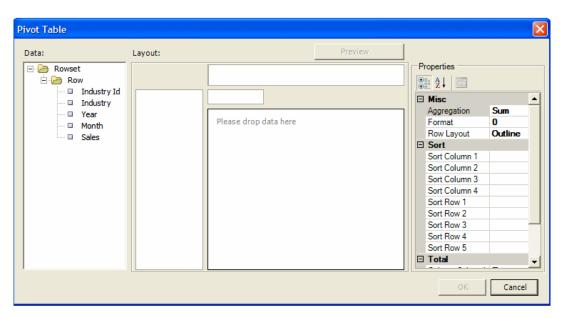
2. Drag and drop the elements from the Data pane to the Layout pane to build the pivot table structure. In the following figure, the layout shows Sales by Industry accumulated by Year and by Month:
