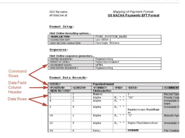
Blank rows can be inserted anywhere in a table to improve readability. Most often they're used in the setup table, between commands. Blank rows are ignored by Publisher when the template is parsed.
