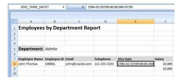
If you do nothing else, the HIRE\_DATE value is displayed as shown. To format the date as "3-Feb-96", you must apply a function to that field and display the results in a new field.
