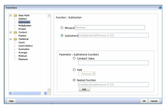
6. Click OK to close the Function dialog. The table column displays the custom formula. Edit the table column header label, and now the table displays the custom function, as shown in the following figure:
