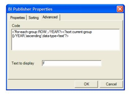
6. When you've completed the dialog options, click **OK**. This inserts the form fields in the template. By default, the beginning for-each form field displays the text "F" and is inserted at the beginning of the selected template section. At the end of the selection, an "E" form field is inserted to denote the end of the repeating group.
