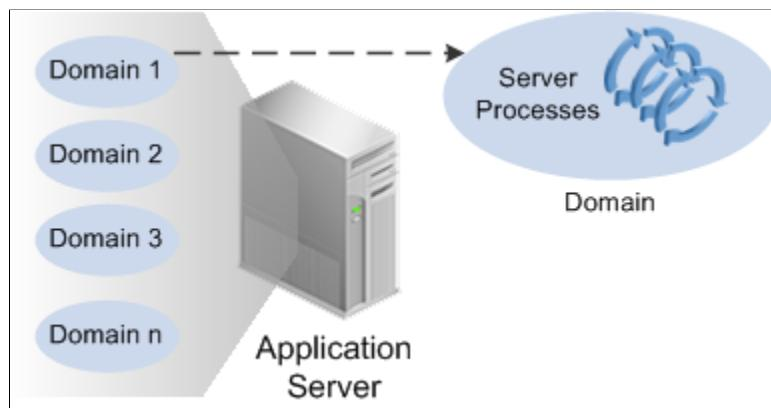
To enhance the scalability of your system, you can configure multiple domains on a single application server machine, and you can also incorporate multiple application server machines to meet the demands of your system.
