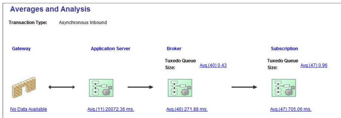
The flow of the transactions are from left to right. In this case you are viewing inbound asynchronous processes, therefore the integration gateway receives the requests and sends the Jolt requests to the application server. The broker evaluates the subscription contracts, and then subscription processing takes place.
