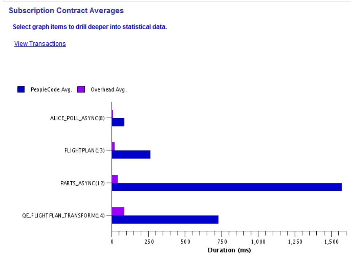
The Subscription Contract Averages page depicts subscription processing times in graphical format. In this example, the bar chart shows the average time for PeopleCode processing and overhead processing for the service operations *ALICE\_POLL\_ASYNC*, *FLIGHTPLAN*, *PARTS\_ASYNC*, and *QE\_FLIGHTPLAN\_TRANSFORM*. The number in parentheses next to each service operation name is the number of transactions involving that service operation reflected in the data.
