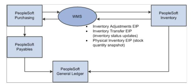
The following diagram shows the process flow for four-wall EIPs in a WMS integration.
