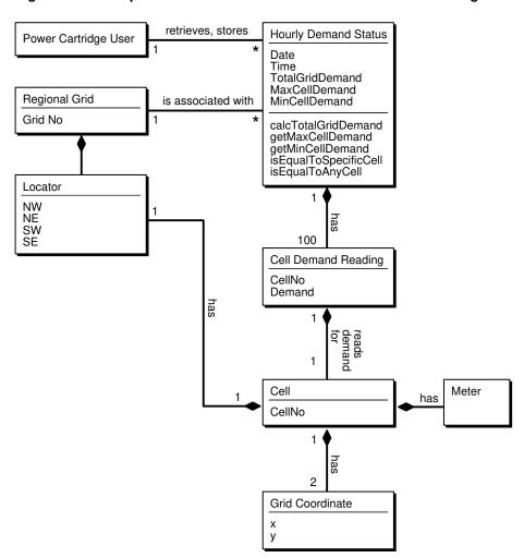
Figure 15-9 Implementation Model of the Power Demand Cartridge
