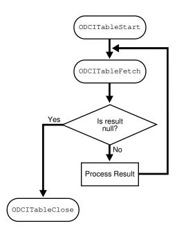
Figure 13-3 Flowchart of Table Function Row Source Execution
