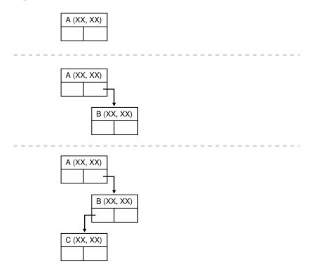
This structure is good at range queries. That is, if the user specifies a point (xx, xx) and a distance, the query returns the set of all points within the specified distance of the original point.
