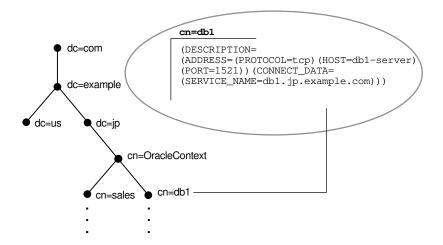
Each entry is uniquely identified by a distinguished name (DN). The DN indicates exactly where the entry resides in the directory server hierarchy. The DN for db1 is dn:cn=db1,cn=OracleContext,dc=jp,dc=example,dc=com. The DN for sales is dn:cn=sales,cn=OracleContext,dc=jp,dc=example,dc=com. The format of a DN places the lowest component of the DIT to the left, then moves progressively up the DIT.
