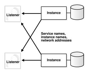
If the listener is not running when an instance starts, then the LREG process cannot register the service information. LREG attempts to connect to the listener periodically, but it may take up to 60 seconds before LREG registers with the listener after it has been started. To initiate service registration immediately after the listener is started, use the SQL statement ALTER SYSTEM REGISTER. This statement is especially useful in high availability configurations.
