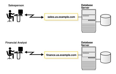
The sales and finance databases are each identified by a service name, sales.us.example.com and finance.us.example.com, respectively. A service name is a logical representation of a database. When an instance starts, it registers itself with a listener using one or more service names. When a client program or database connects to a listener, it requests a connection to a service.
