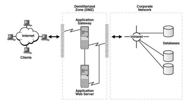
It is important to deploy at least two Oracle Connection Manager firewalls or Oracle Net Firewall proxies in an Internet network environment in the event that one firewall goes down.
