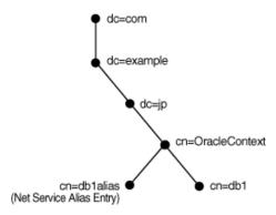
There are several uses for network service aliases. As shown in Figure 3-9, a network service alias can be useful as a way for clients to refer to a network service name by another name. Another use is to have a network service alias in one Oracle Context for a database service or network service name in a different Oracle Context. This enables a database service or network service name to be defined once in the directory server, but referred to by clients that use other Oracle Contexts.
