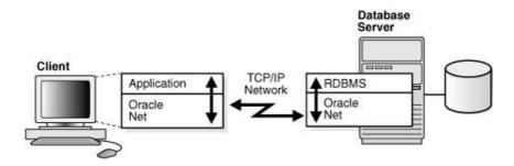
Specifically, Oracle Net is comprised of the Oracle Net foundation layer, which establishes and maintains connections, and Oracle protocol support, which maps the foundation layer technology to industry-standard protocols.
