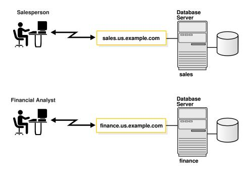
Instances are identified by an instance name, such as sales and finance in this example. The instance name is specified by the INSTANCE\_NAME initialization parameter. The instance name defaults to the Oracle system identifier (SID) of the database instance.
