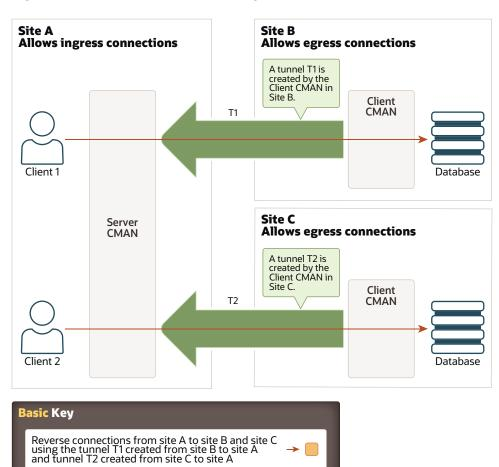
Figure 5-8 Reverse Connection Using CMAN Tunnels
