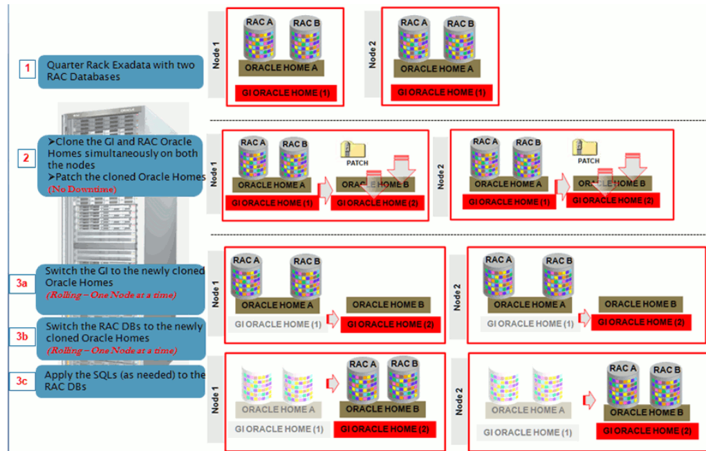
Figure 43-10 Out Of Place Patching Of Clusters
