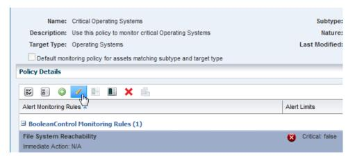
**3.** Edit the rule parameters. In this example, the default time to generate an alert is changed from 10 minutes to 5 minutes.
