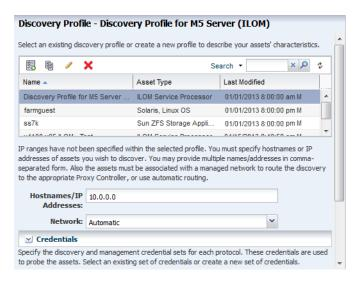
**5.** Enter the host name or IP address for the server's service processor, then click **Add Now** to launch the discovery job. You can also discover multiple servers using an IP range. This might take a few minutes to complete.
