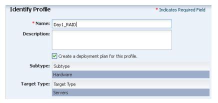
**4.** Enter a name for the volume and choose its RAID level. Your options for RAID level depends on the number of available disks. The default RAID level, RAID0, is not recommended.
