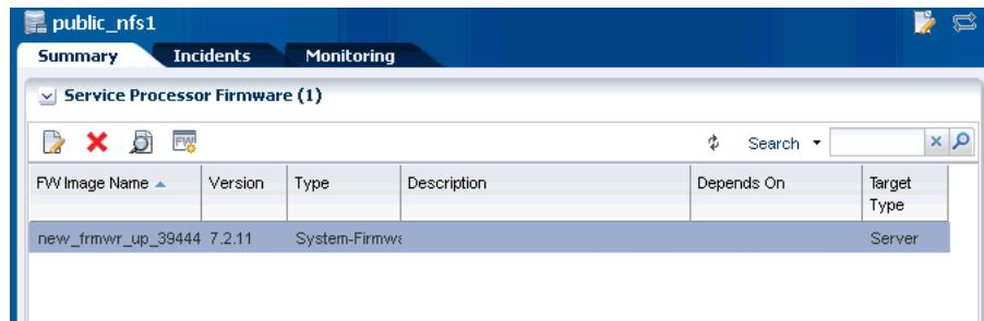
When you upload a firmware image, a default firmware profile and deployment plan is automatically created.
