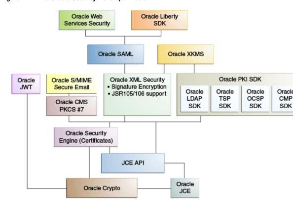
Figure 1-2 shows the components of the Oracle Security Developer Tools. Typically, a tool will utilize functions provided by the tool immediately below it in the stack. For example, the Oracle SAML tool leverages functions provided by the Oracle XML Security tool.
