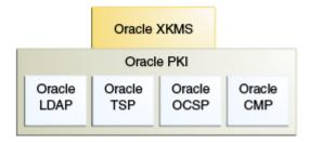
This graphic shows that Oracle's XKMS tool is built on Oracle PKI tools, which consist of Oracle LDAP, Oracle TSP, Oracle OCSP, and Oracle CMP.
