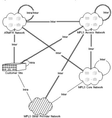
Figure 24 MetaSolv TM MPLS Network Template
