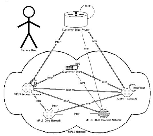
Figure 25 MetaSolv TM MPLS VPN Network Template
