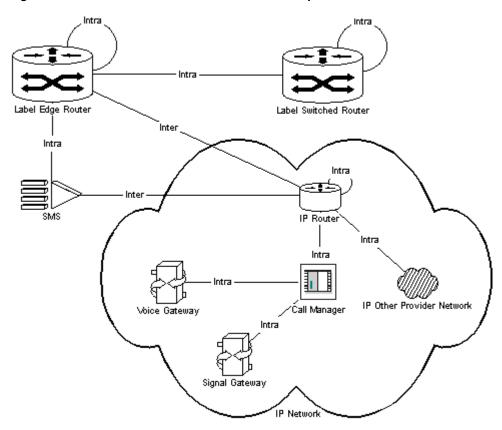
Figure 24 illustrates the MetaSolv TM MPLS network template.
