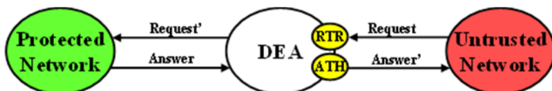
Figure 16: Diameter Topology Hiding Trigger Points: Untrusted-to-Protected Transactions
