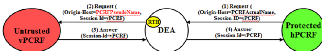
Figure 32: Protected-hPCRF to Untrusted-vPCRF Transaction
