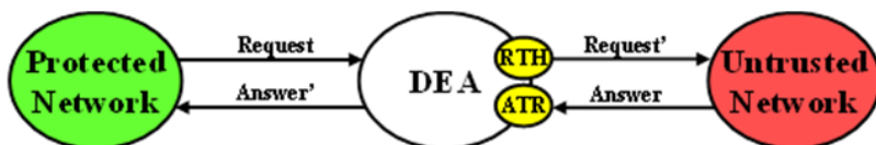
Figure 15: Diameter Topology Hiding Trigger Points: Protected-to-Untrusted Transactions
