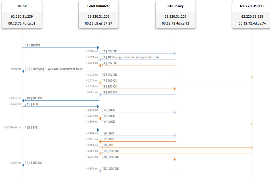
Figure 4–18 Example Call Flow
