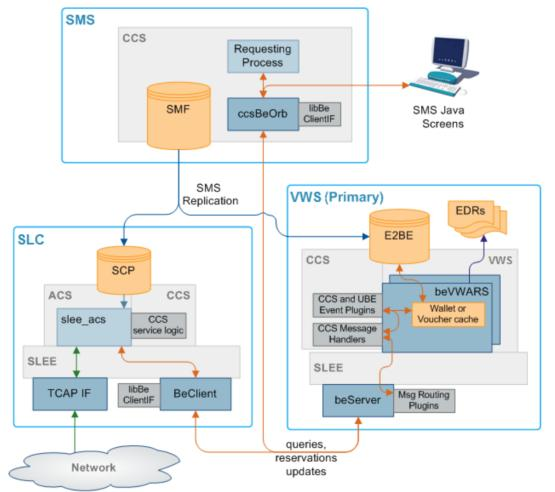
Here is an example of how the VWS handles requests from CCS on an SLC to a VWS.
