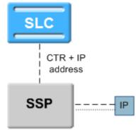
**3** The SLC communicates with the SSP through the ETC (EstablishTemporaryConnection) and IP address. The SSP then uses the IP address to communicate with an external IP.
