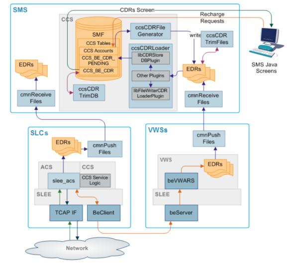
Here is an example showing EDR creation, transfer to the SMS and processing.
