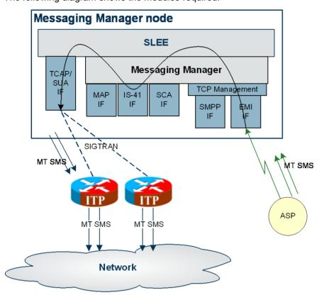
The following diagram shows the modules required:
