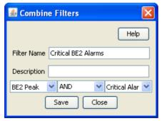
2 In the **Filter Name** field, enter a name for the filter.
