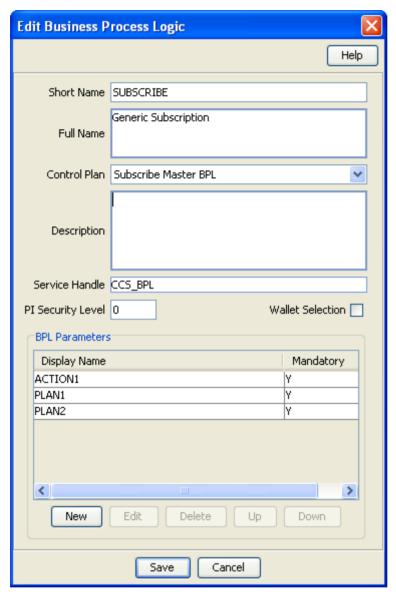
When the command is run via the PI, it will trigger the specified Service and Control Plan, which will handle the complicated interaction required, and set a response code using a Cause Value inside a Disconnect node in the associated Control Plan. Calling BPL is done using the command CCSBPL=EXE. For example:
