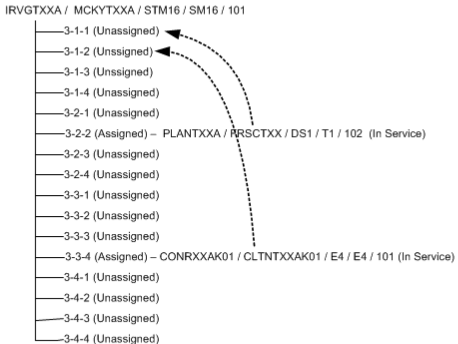
Figure 14-25 Intra-Facility Grooming: Required Changes
