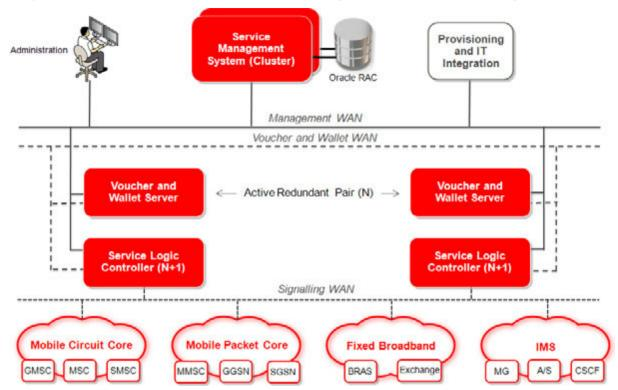
Note: The configuration of the VWS in a redundant pair set-up and the SLC running in an N+1 configuration. Here the SMS is set up in a redundant cluster configuration using Oracle RAC for the database component.
