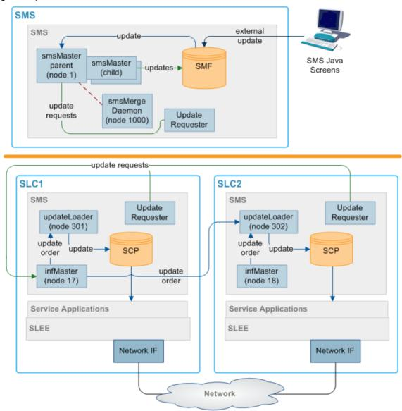
Where the master is isolated from the network, each update loader looks for the inferior master with the lowest node number and connects to that.
