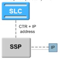
The SLC communicates with the SSP through the ETC (EstablishTemporaryConnection) and IP address. The SSP then uses the IP address to communicate with an external IP.
