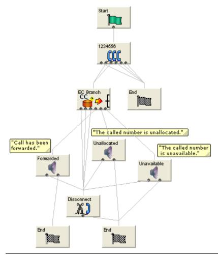
You would set up the configurable exits of the branch on ERRB Cause Code node as shown below.
